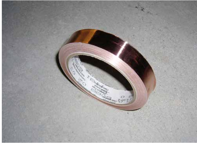
2 Copper strip (self-adhesive) used to produce antistatic floor covering.
